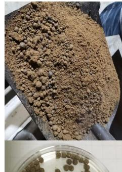
□Unevenly conditioned, water resistance failure rate of 24%
